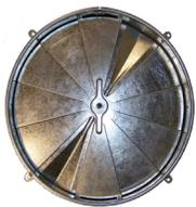
**Radial Bow tie Damper** - Facilitates accurate airflow modulation and control using a linkage that is tight and vibration free. It has low torque operation through the entire range of adjustment. This damper is riveted to the Pharmaseal housing.
