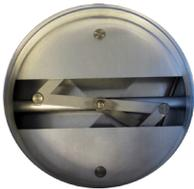
**Guillotine Damper** - This damper facilitates room balancing and airflow control. It is easily adjusted using the 1/4-turn rotary mechanism attached to a robust mechanical linkage and heavy-duty blades. The damper assembly is welded to the hood body to increase rigidity and eliminates "binding" of damper blades common in pop-riveted units.
