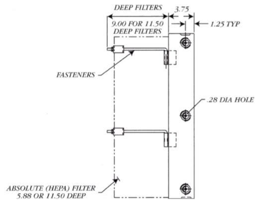
equi-bearing clamps to allow uniform filter sealing.
