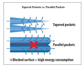
Camfil Hi-Flo pocket filters operate more efficiently and last longer because of their tapered pocket stitching. Incorporating the same amount of media relative to competitive bag filters, minimizing configuration losses and product engineering make the difference.
