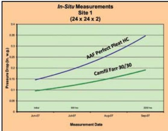
The Camfil 2" deep 30/30® outperformed the American Air Filter® PerfectPleat® by a factor of over two to one. Since this was a constant volume system that adjusts for changes in pressure drop, the energy saved by using the 30/30 in this application is significant.
