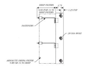
equi-bearing clamps to allow uniform filter sealing.
