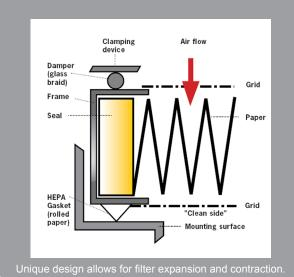
Incorporating a unique, floating component design, the Camfil Termikfil Absolute maintains integrity and rated performance values in applications where extremely high temperatures are a factor. Pre-qualified with an exclusive burn-in procedure, which significantly reduces system start-up time, the Termikfil outperforms other high-temperature filters.
