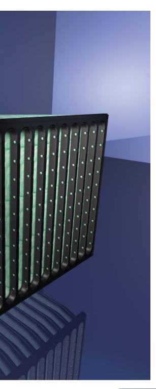
The reinforced ABS plastic header frame is assembled from matching halves to provide rigid and durable filter support. Frame racking is eliminated and the filter fits securely into the side-access housing or built-up bank holding frame. Its rigidity reduces the possibility of air bypass, even during turbulent airflow. One vertical header includes a gasket to prevent air bypass between filters when they are installed in a filter track.
