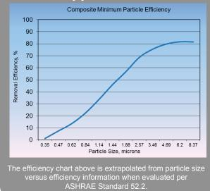
The Camfil Farr Aeropleat<sup>®</sup> III pleated filter offers medium grade ASHRAE efficiency, and sets the performance standard for those upgrading from lower efficiency pleats, throw-aways or pads. The Aeropleat III has a MERV 8 when evaluated per ASHRAE Standard 52.2.
