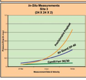
The Camfil 2" deep 30/30 was evaluated at a third facility with similar results. While providing a true MERV 8 efficiency as required by hospital authorities, it demonstrated a long-loading curve indicating that it would have a significantly longer life than the competitor's filters tested. After six months of operation, the 30/30 resistance increased less than 15% indicating that it could easily last a year without taxing the system.
