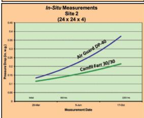
The Camfil 4" deep 30/30 outperformed the Air Guard® DP-40 over a seven-month period with the same results as above. At 10 cents per kWh this system would save over \$20.00 per filter throughout the facility.
